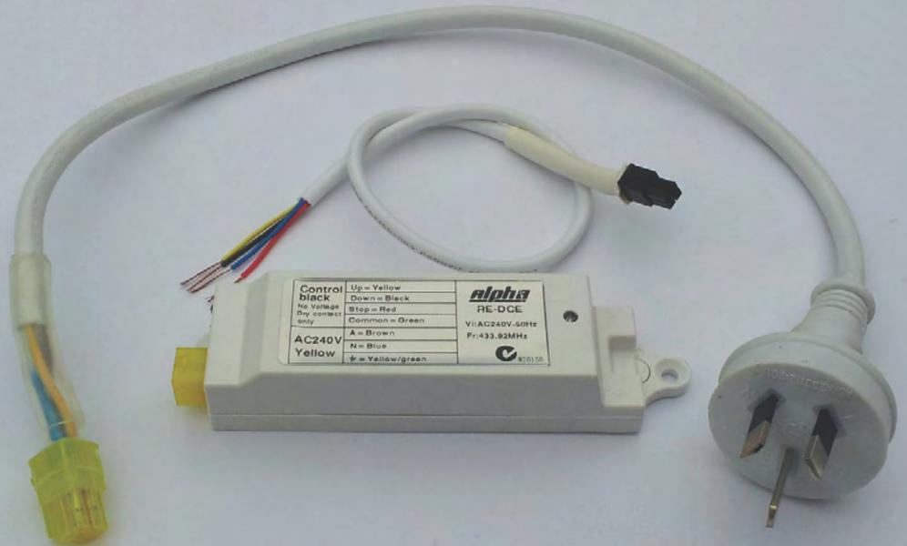
This device is a single channel remote control that plugs into a power point for permanent power and is controlled by connecting the device to relays in a control system or other switches. There are 4 wires connecting this item: common, up, stop and down. When the common wire comes into contact with any of the control wires, the function for that wire will be sent out to any WSER series motors or remote receivers this device is assigned to.
