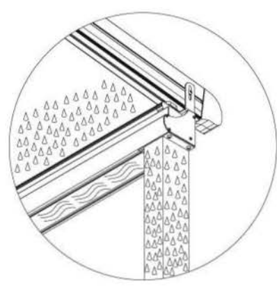
Water drainage details
