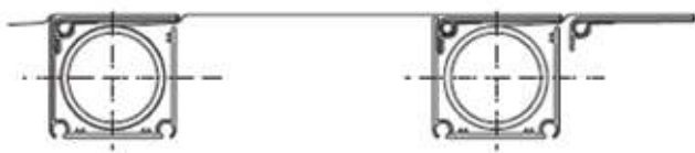
Fabric casing with extended fabric (maximum 1m between windbreaks when extended)
